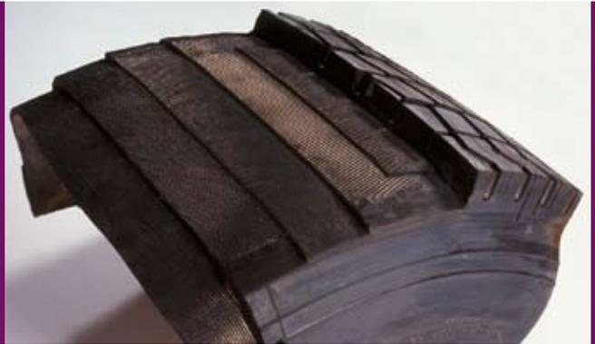
Steel cord for radial tire reinforcement
