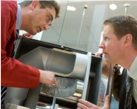
Diesel particulate filter using metal fibers
