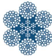
The Diamond Blue is a 6 strand galvanized conventional rope produced with a steel core fully lubricated during production process.
