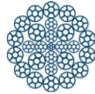
50 DB Series ropes are compacted rotation resistant galvanized constructions consisting of an inner part with an outer layer of strands spun in the opposite direction.
